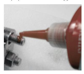
**For Blind Holes**, apply several drops down the female threads into the bottom of the hole. As threads are engaged, compressed air forces the product upwards into the threads.
